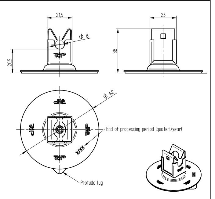
The adhesive area on the smooth surface should be thoroughly cleaned before applying the support for example with isopropylalcohol! Processing temperature +15 to +25°C!
